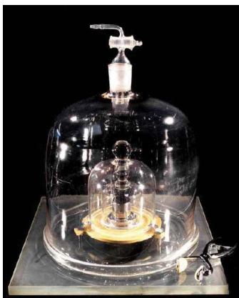
Figure 1.6.1: The Kilogram. The standard for the kilogram is a platinum-iridium cylinder kept in a special vault in France. Source: Photo reproduced by permission of the Bureau International des Poids et Mesures, who retain full internationally protected copyright.
