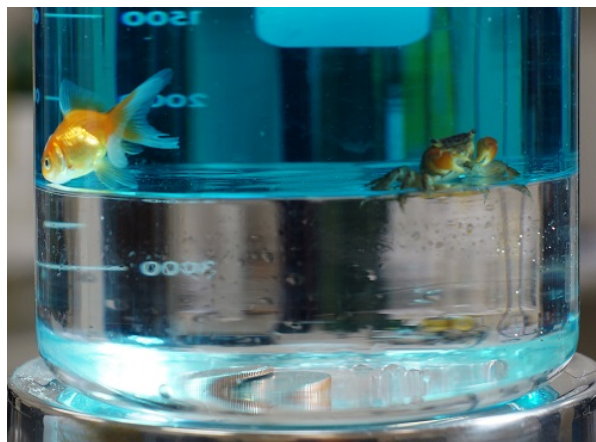
Figure 10.2.1: A beaker holds water with blue food dye (upper liquid layer) and a much more dense perfluoroheptane (a fluorocarbon) lower liquid layer. The two fluids cannot mix and the dye cannot dissolve in fluorocarbon. A goldfish and a crab have been introduced into the water. The goldfish cannot penetrate the dense fluorocarbon. The crab floats at the liquid boundary with only parts of his legs penetrating the fluorocarbon fluid, unable to sink to the bottom of the beaker. Quarter coins rest on the bottom of the beaker. Animals were rescued from their predicament after the photo was taken. Figure used with permission from Wikipedia (Sbharris (Steven B. Harris)).
