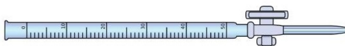
Fig. 12.4.1 Equipment for Titrations. A burette is a type of liquid dispensing system that can accurately indicate the volume of liquid dispensed
